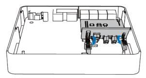
**STEP 3** Insert a SIM card on the GSM/CDMA/3G module following the instructions. Skip this step if no GSM/CDMA/3G module installed.
