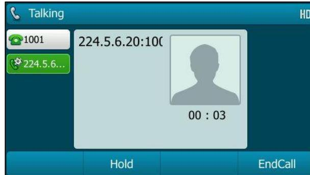
2. To place the current multicast RTP session on hold, press the **Hold** soft key.
