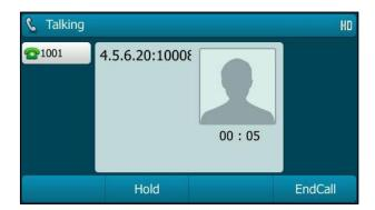
4. To place the current multicast RTP session on hold, press the Hold soft key.
