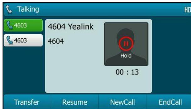
The line key LEDs on phone A slow flash green and phone B slow flash red when the shared line call is placed on hold.
