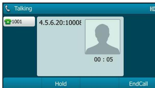
4. To place the current multicast RTP session on hold, press the **Hold** soft key.
