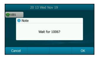
Press the **OK** soft key, the phone returns to the idle screen and call completion is activated. When the called party becomes idle, the LCD screen prompts the following:
