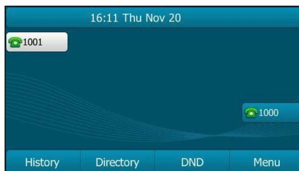
When you assign functionality to line key located in line key 11-27, the label of the line key 10-18 are indicated on the second page, and the labels of the line key 19-27 are indicated on the third page. The line key in the right bottom is used to switch pages. The following figure shows an example:
