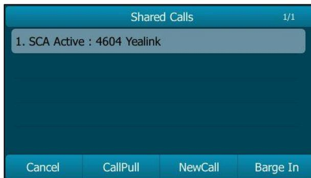
2. Press the **Barge In** soft key to interrupt the active call of phone A.
