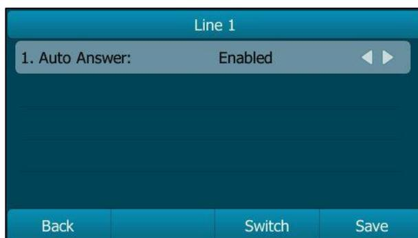
4. Press the **Save** soft key to accept the change or the **Back** soft key to cancel. The **AA** icon appears on the LCD screen.
