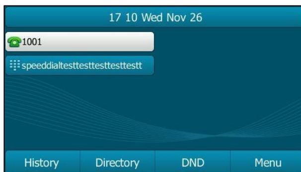
The following figure shows an example of label display when the label length feature is disabled:
