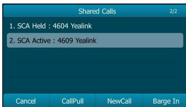
3. Press the **Barge In** soft key to interrupt the active call of phone A.
