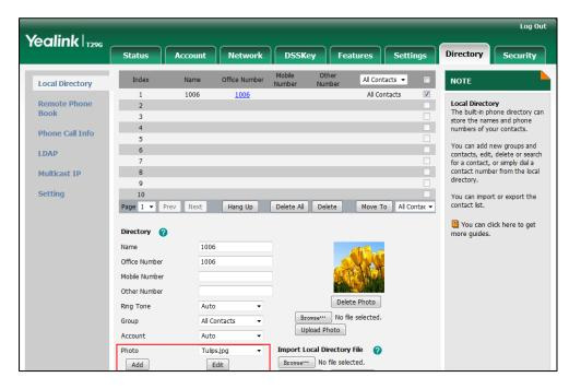
When you place a call to the contact or receive a call from the contact, the LCD screen will show the contact photo.
