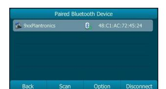
The LCD screen displays a list of paired and connected Bluetooth headsets.
