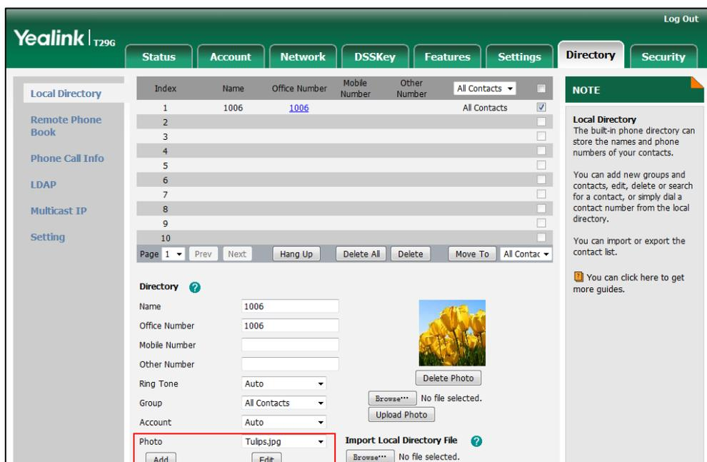
When you place a call to the contact or receive a call from the contact, the LCD screen will show the contact photo.
