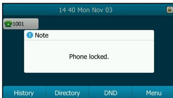
To unlock the phone, you must know the phone unlock PIN. The default phone unlock PIN is "123".
