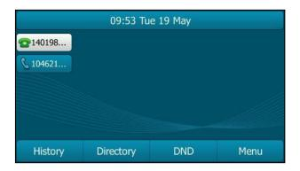
Any IP phone can be used to originate or receive calls on the bridged line. An incoming call to the BLA number can be presented to multiple phones in the group simultaneously. The incoming call can be answered on any IP phone of the group but not all.
