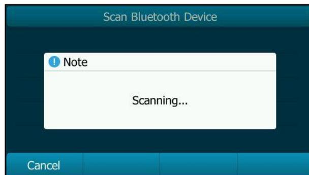
The phone proceeds to scan the local Bluetooth devices. When the phone completes scan, it will display the found Bluetooth devices on the LCD screen.
